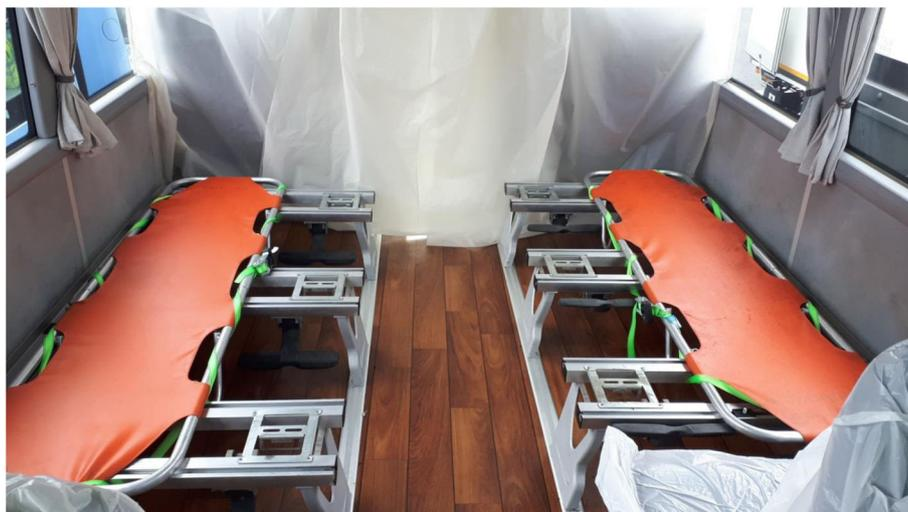
**Fig. 2** Two workstations in the "contaminated" area at the rear of the CCCA. The vertical vinyl film (seen in the back) creates a separation from a "clean" area located at the front of the bus, including the driver's compartment and a rest area
