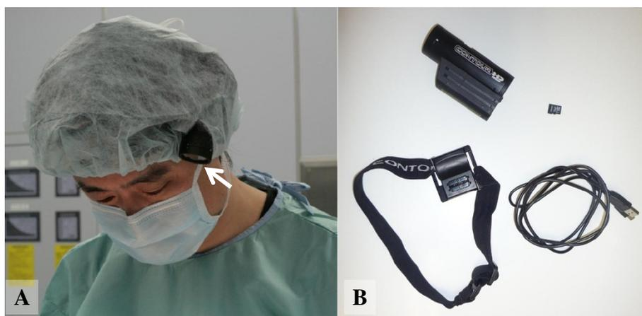
**Figure 1** Commercially available head-mounted camera (ContourHD, Contour Inc., Seattle, Washington, USA.). **A:** We wear the camera (white arrow) under a surgical cap. Because the device is cordless, video recording can be quickly and easily prepared. **B:** The equipment used in our study is shown. It comprises (clockwise): the head-mounted camera; 16GB microSD card; USB cable for transferring digital data to a computer; elastic headband camera mount.
